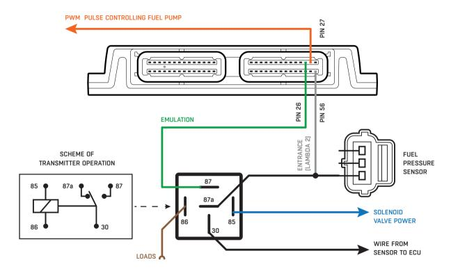
**NOTE!** The original controller wiring is not equipped with a cable for the PWM signal (pin27) connection and the emulation output cable (pin26). Wiring for emulation pressure and the pressure emulation transmitter are available optionally as ELE00126 Pressure Emulation Set OPTIMA EXPERT. The set consists of 2 wires and transmitter.
