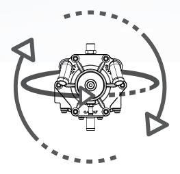
Because there is no integrated solenoid valve and liquid phase filter, the reducer can be installed in any position, however, we recommend installation with the gas outlet downwards.
